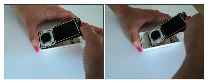
• Using your fingers, gently pull the top of the circuit board up toward you while also sliding the bottom of the circuit board away from the bottom of the Sirius Stiletto 100 back cover.
