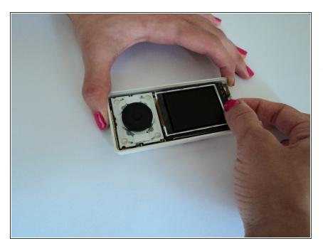
While looking down at the device, place your index finger at the top of the circuit board and your thumb on the device screen.
