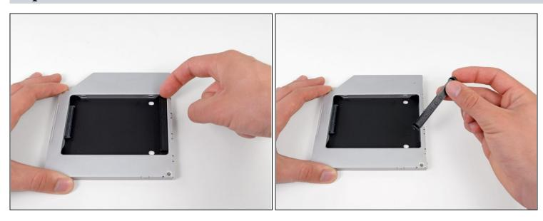
• Remove the plastic positioner from the optical bay hard drive enclosure by pressing in on one of the clips on either side and lifting it up and out of the enclosure.
