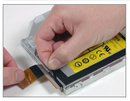
Peel up the black tape partially covering the orange optical drive cable.
