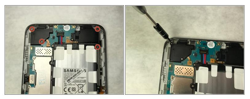
• Using a phillips head screwdriver, remove the two 4mm screws holding down each speaker.
