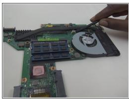
• Use a Phillips screwdriver to loosen the four screws holding the component in place.
