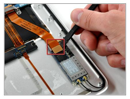
Using a spudger, pry the AirPort/Bluetooth ribbon cable connector straight up off the AirPort/Bluetooth board.
