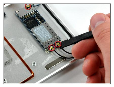
Use a spudger to pry the three antenna cables up off the AirPort/Bluetooth board.
