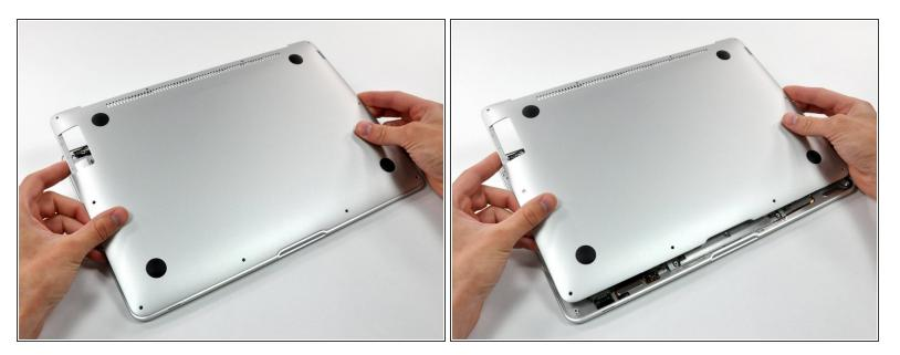
Slightly lift the lower case near the vents and push it toward the rear of the computer to free the mounting tabs.
