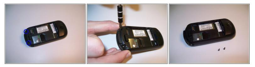
• Use a Torx T-5 screwdriver to remove the screws on the back of the phone.
