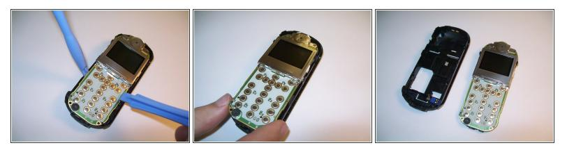
• Use plastic opening tools to free the circuit board from the case.
