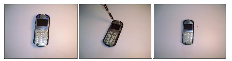
• Using a Torx T-5 screwdriver remove the screws at the top of the phone.
