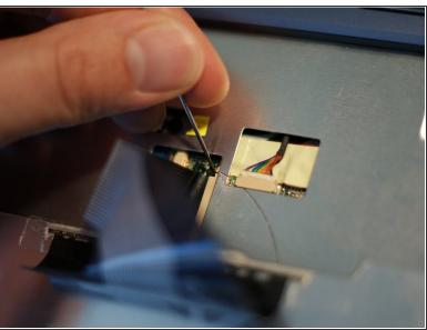
• The keyboard is connected with a flat cable. At the socket, push the black bit below the cable away from the socket (in the direction of the cable) and pull the cable out. I found the 1 mm round bit useful for this, but a needle works fine as well.
