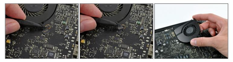
• Use the tip of a spudger to lift the left fan connector straight up from its socket on the logic board.
