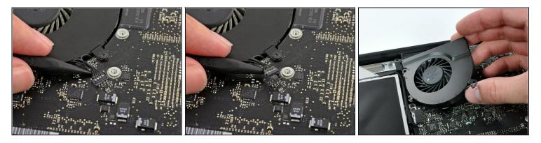
• Use the tip of a spudger to lift the right fan connector straight up from its socket on the logic board.
