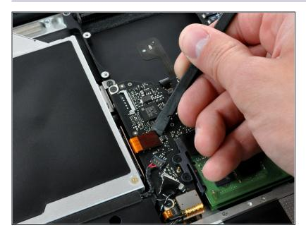
Use a spudger to carefully pry the optical drive connector straight up off its socket on the logic board.
