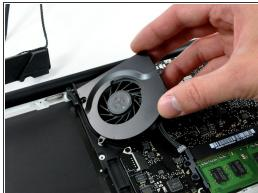
A connector, three Phillips screws, and bam -- the fan's out!
