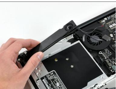
The subwoofer comes off after removing two screws.
