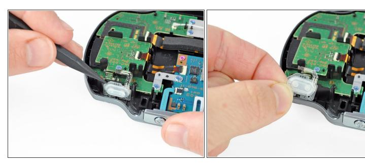
Using a spudger, gently peel up the left shoulder button from the light adhesive connecting it to casing.
