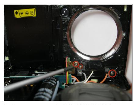
Unscrew the three 3x2mm screws that attach the cables to the front casing.
