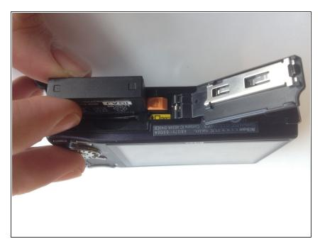
Slide the orange switch to the right as shown. Now the battery can be pulled out. Reverse these steps to re-install.
