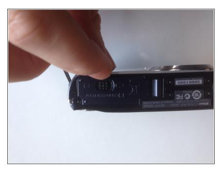
On the bottom right of the camera, locate the battery flap switch.
