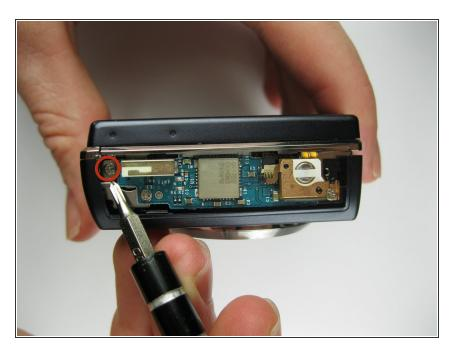
Remove the 3x2mm screw underneath the panel near the top of the camera.
