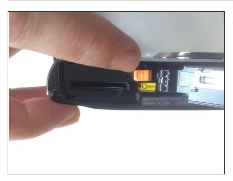
Move this switch to the right so the battery flap can flip open.
