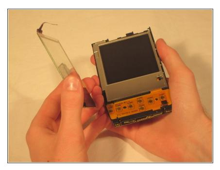
Reinsert the screen into the case that contains the buttons.
