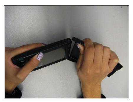
Gently snap the flip cover back into place where it connects at the top of the Palm IIIc
