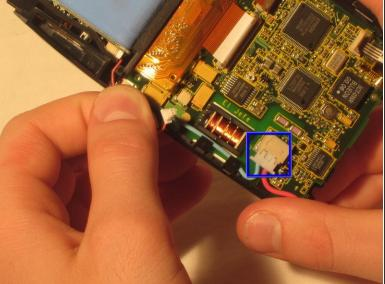
Connect the blue and red screen cables to the beige box they were removed from.
