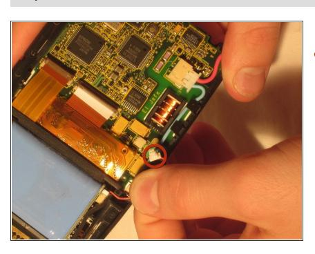
Attach the white box on the end of the red cable connected to the battery into the connector box on the motherboard.
