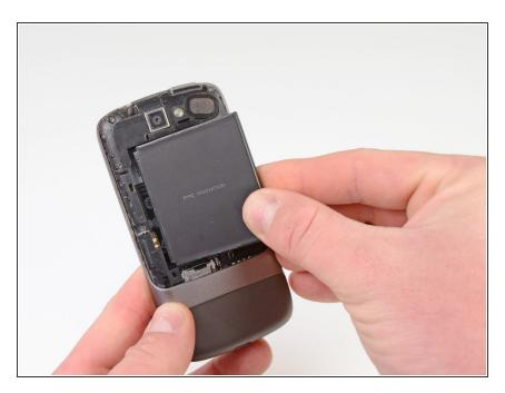
• Pull the battery up and out.
