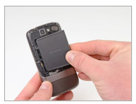
Pull the battery up and out.
