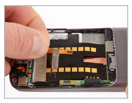
Pull up on the ribbon cable, the tape will detach from the main board ribbon.
