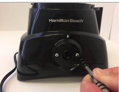
Remove the two 11 mm screws using the #2 Phillips head screwdriver.
