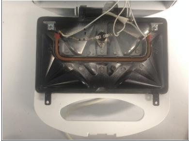
Remove the mold to get access to the heating coil.
