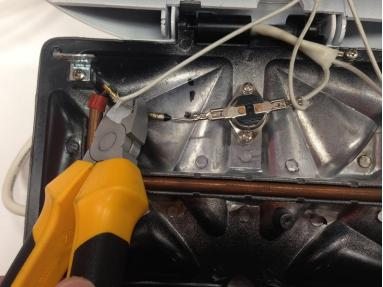
• Cut the two wires that connect to the thermal fuse.
