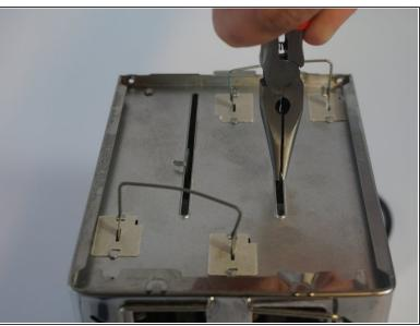
Using the needle nose pliers, bend the two metal strips so they are facing the same direction.
