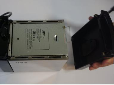
Remove the black casing by sliding it upwards.
