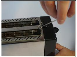
Remove the two wire frames located on top of the toaster.
