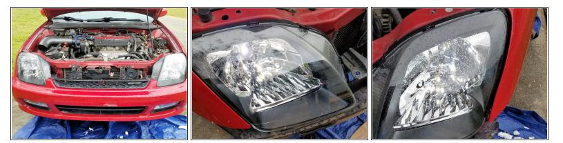
Follow the disassembly steps in reverse to secure the new headlight assembly. Take care to use the same bolts that were removed and replace any missing bolts with stock body screws from an auto parts store.
