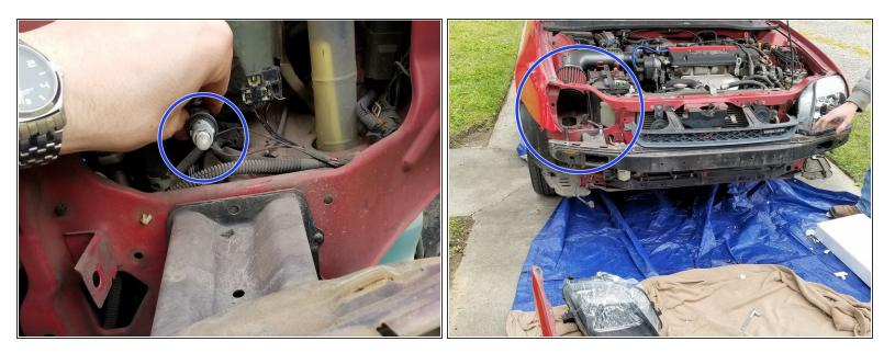
When removing the headlight, take care to avoid touching any bulbs with your hands or wear a latex glove. Furthermore, do not force the assembly to come out. If the assembly does not come free with a gentle pull then something is likely still attached.
