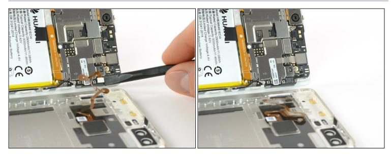
• Disconnect the fingerprint sensor using a spudger.
