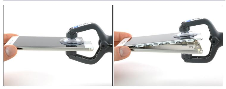
Avoid to lift only the display instead of the whole phone assembly as doing so may cause damage to the screen.
