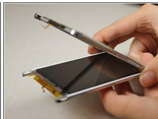
**⚠ Warning:** If you are too rough with the screwdriver, you can permanently damage the display.
