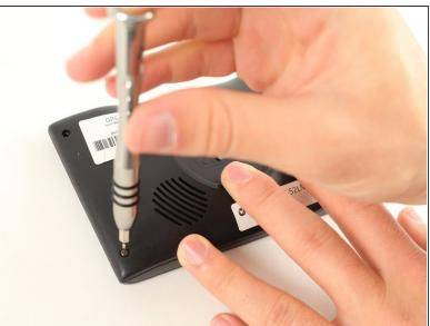
Place the device face-down, with the screen facing the surface. There are 8.7mm screws located
