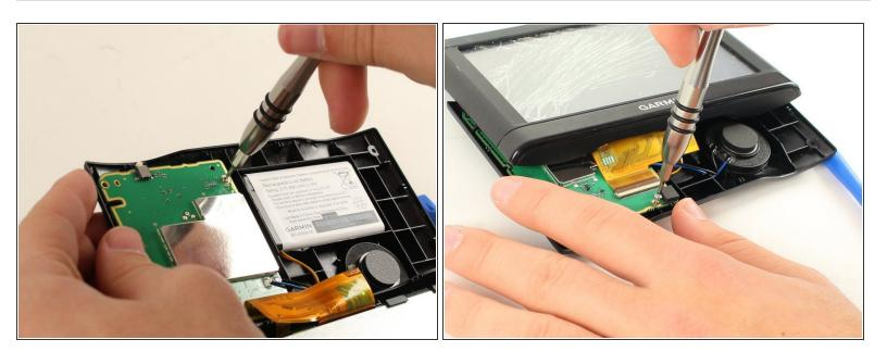
Using the T5 Torx screwdriver, unscrew the two 5.6mm screws at the top right and bottom right corners of the motherboard.
