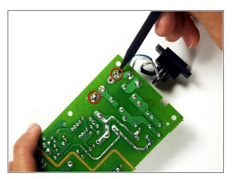
Desolder the items circled in red from the first circuit board you removed.
