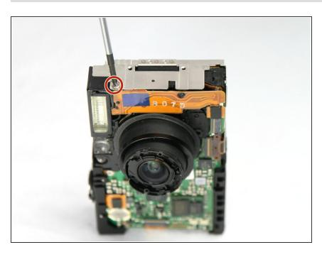
Use a Phillips #00 screwdriver to remove the 2.4 mm screw that secures the flash assembly.
