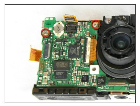
Remove the two 2.90 mm screws from the motherboard.
