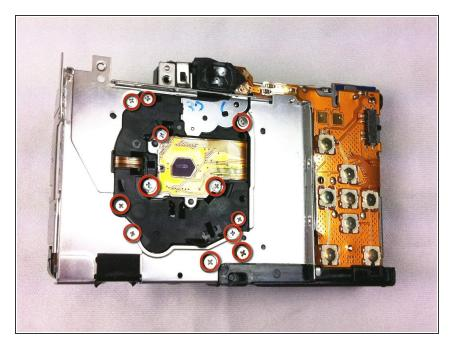
Remove the screws shown. Start with the outside 6 (3-2.90mm & 3-2.40mm) screws on the metal frame. Then remove the 6 (2.40mm) screws on the back of the lens piece
