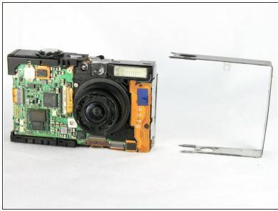
Slide the metal frame off of the camera on the side that is closest to the flash mechanism.
