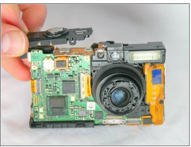
• Using the spudger, take off the shutter button by prying the small tab on the front side of the camera.
