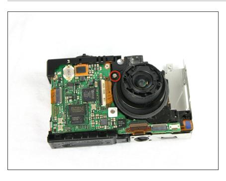
Remove the 2.90mm screw from the lens, near the motherboard.
