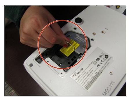
Remove the light bulb from the projector by lifting the silver handle and pulling up.
