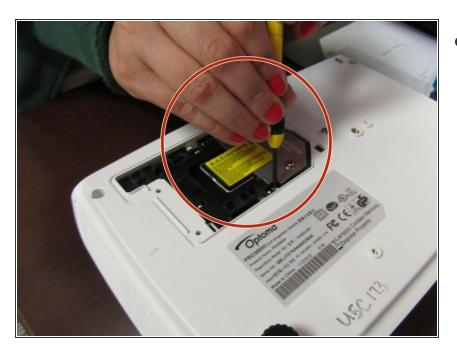
Unscrew the bulb screws on either side of the silver plate.
