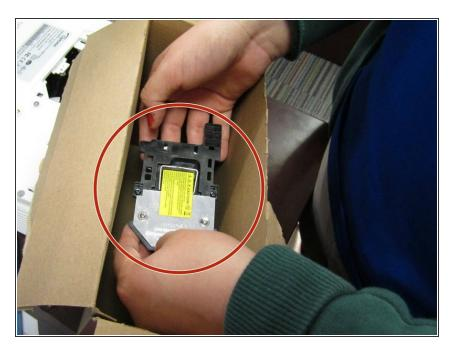
Open and remove the new light bulb from its box with clean hands to prevent from getting the bulb dirty.
