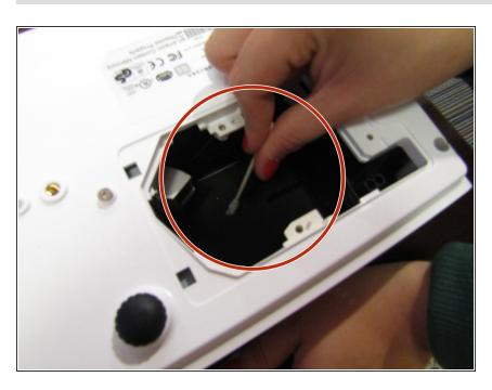
Clean the now vacant area where the light bulb once belonged of dust and particles using a Q-tip.
