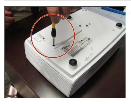
On the bottom side of the projector, locate and unscrew the back cover using a Philip's head screwdriver.
