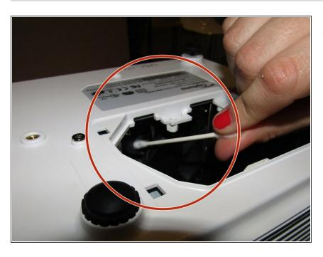
Use a new Q-tip to clean the fan blades and hole in which the light enters.
