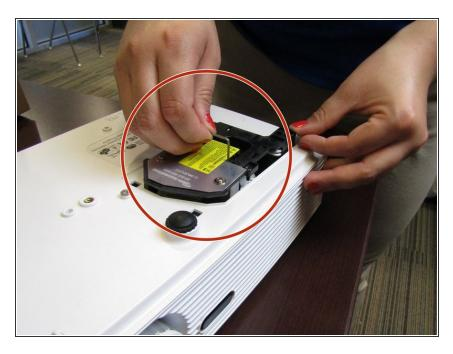
Place the new bulb inside making sure to align the bulb towards the light hole and the wire connector towards the wire receiver.
