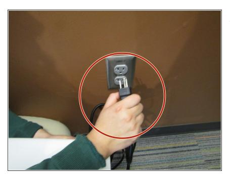
Unplug the projector from the wall outlet to allow for the light bulb to cool for at least 30 minutes.
