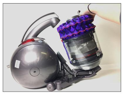
• Remove the canister by lifting it out.
