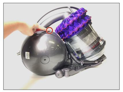
Press the gray button to release the canister.
