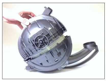
Remove the bottom half of the plastic sphere to reveal the motor.
