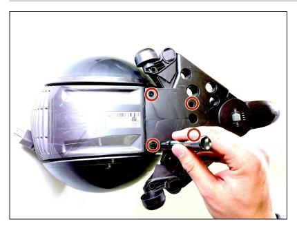
Find and remove the four 21.5mm screws on the bottom that hold the base plate on using a T15 Torx bit.
