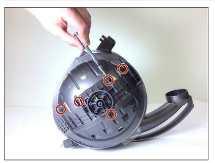
Locate and remove the five 22mm screws on each side of the ball that keep the plastic enclosure together using a T15 Torx bit.
