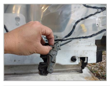
Remove the end of the cable out of its location.
