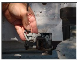
Insert your hand inside the bottom of the door to retrieve the door latch.
