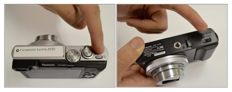
• Turn the camera off and identify the battery door located on the bottom of the camera.
