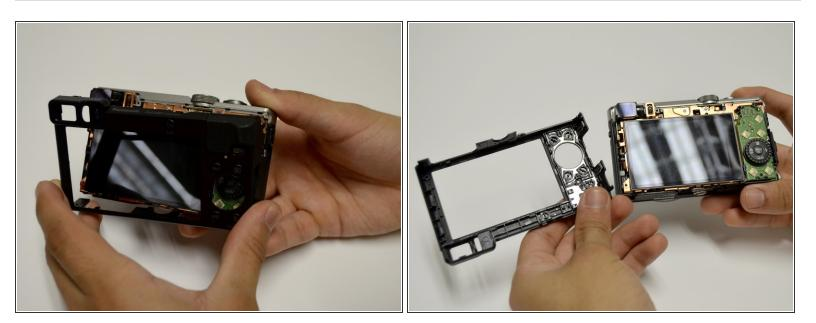
• Remove the casing from the camera by hand or using a plastic opening tool.
