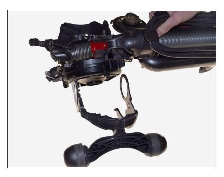
After the final screw is removed, pull off the wheels on both sides of the vacuum.
