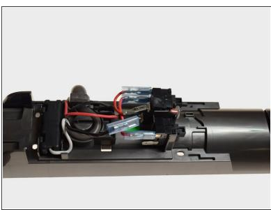
Remove the black wire from its connection near the top of the hatch
