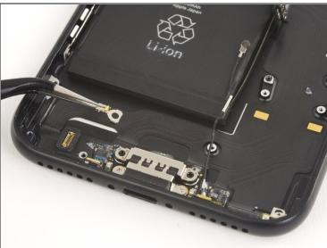
• Remove the spring contact from the lightning connector.
