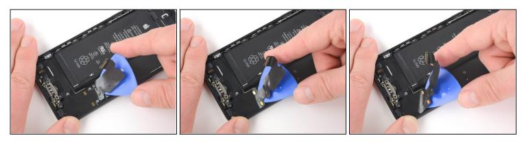
• Continue to slide the pick towards the lightning connector to further separate the assembly from the rear case.
