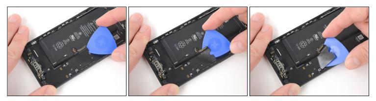
• Starting from the middle of the phone, slide an opening pick underneath the lightning connector to separate it from the rear case.
