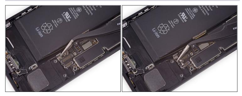
• Use tweezers to derout the antenna cables from their bracket on the logic board.
