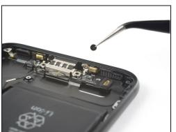
• Remove the two stickers covering the screws that secure the lightning connector to the bottom of the rear case.
