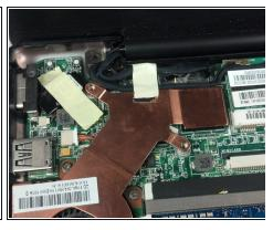
• Peel the foam adhesive pad off from the top of the copper plate, as well as the tape located beneath that.
