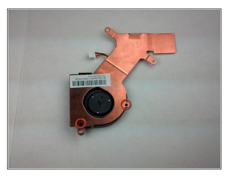
Use a Phillips #0 screwdriver to remove the two 2.35 mm screws securing the fan to the copper plate.
