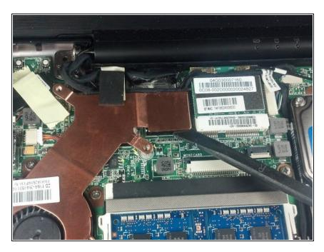
Slide the spudger under the righthand edge of the copper heat sink in order to disconnect it from the thermal pad below.
