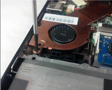
• Use a Phillips #0 screwdriver to remove the two 3.76 mm screws securing the fan/heat sink assembly to the motherboard.
