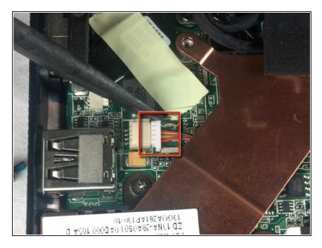
Using the spudger, gently push at the top and bottom ridges of this wire bus to disconnect it from the socket.
