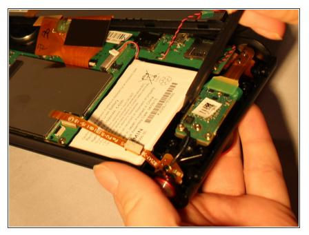
• Locate the white box in your device which is the battery.
