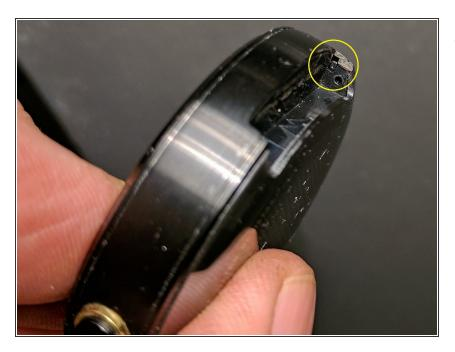
Locate the rectangular end of the fastener inside the wrist strap mounting pocket.
