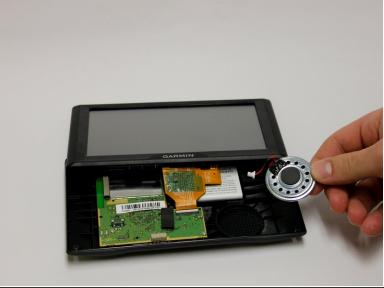
Using a plastic spudger and your fingers, remove the speaker from the device.
