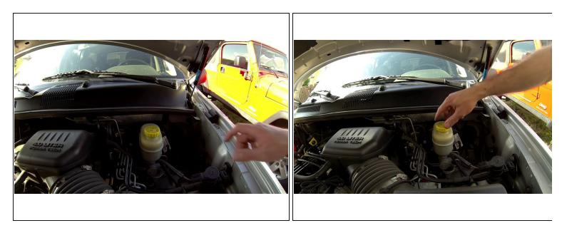
• Open the hood and locate the brake fluid reservoir at the back of the engine compartment
