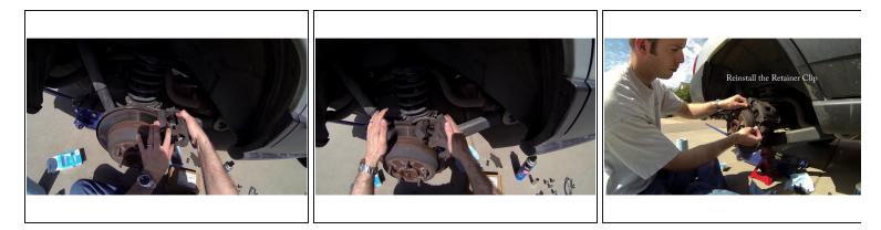
• If the brake piston is not retracted enough to allow for the additional width of the new thicker brake pads, installing the brake caliper can be more difficult
