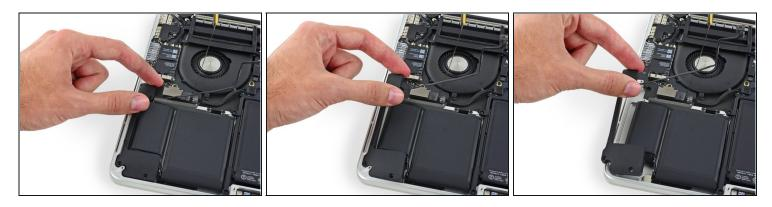
• Lift the right speaker from the cable end and pull it free from the case.
