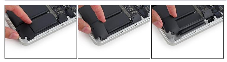
• Lift the corner of the left speaker up and slide it out around the battery to remove it from the upper case.
