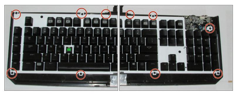
Using the Phillips #0 Screwdriver, remove the ten 10mm screws that are indicated by the red markers.
