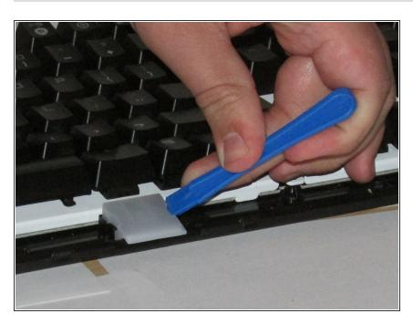
Using a plastic opening tool, lift the plastic covering away from the LED light.
