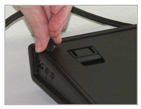
Gently pull off the four rubber tabs located on the corners of the keyboard with your fingers.
