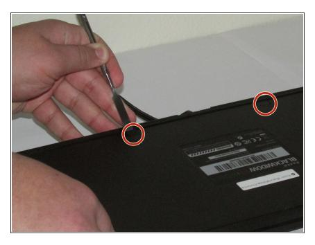
Using a metal spudger, gently remove the plastic tabs that are covering the two screws.
