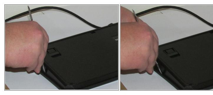
Using a metal spudger, begin prying off the faceplate of the keyboard. There are small tabs along the edge of the keyboard and the faceplate that must be released. There are four tabs along the front of the keyboard and two along each side.
