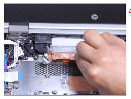
Carefully peel back the foil as necessary to free the speaker cable from the base of the laptop.
