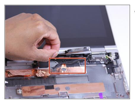
Remove the cable from its routing path.
