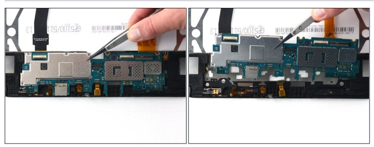
• Use nylon-tipped tweezers to remove the motherboard.
