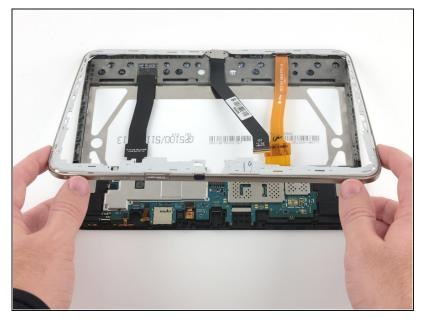
• Lift the plastic frame to remove.
