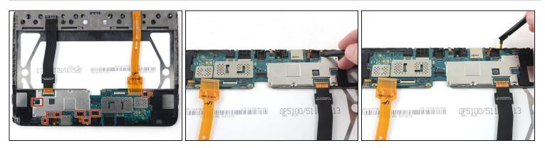
Use a nylon spudger to flip up the eight press-fit connectors from the motherboard.
