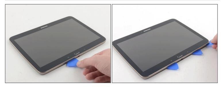
• Insert an opening pick between the rear case and the plastic rim.
