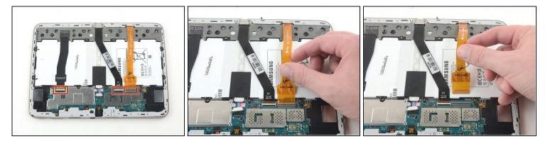
• Remove all three ribbon cables by gently pulling the cables away from the ZIF connectors.
