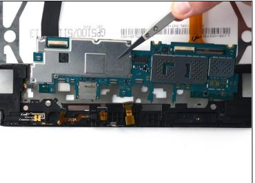
• Use nylon-tipped tweezers to remove the motherboard.
