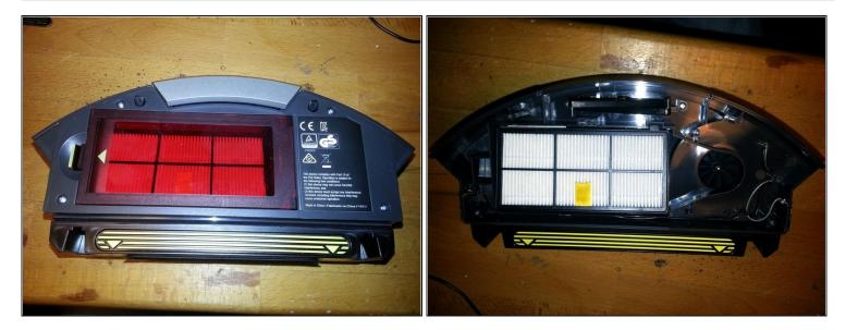
• Open the lid of the vacuum bin by removing the four silver screws and carefully remove the lid
