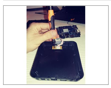
Using your Phillips head screwdriver remove the 2 screws that hold the unit to the housing
