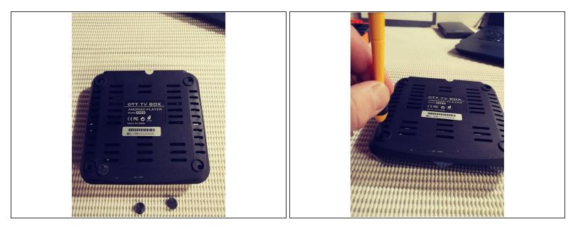
• Remove 4 circle pads to access the 4 screws. Using a Philips head screwdriver, remove all 4.
