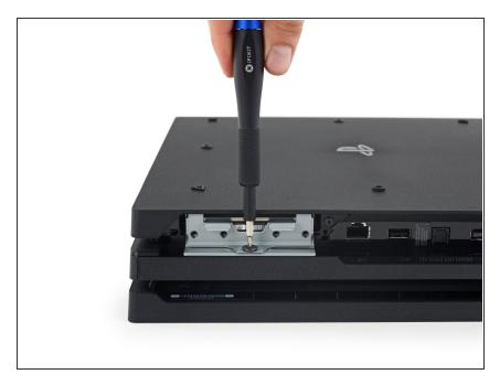
Remove the Phillips #0 screw securing the hard drive caddy to the chassis.
