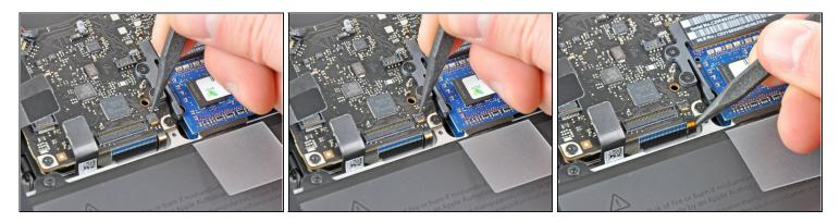
• Use the tip of a spudger or your fingernail to flip up the retaining flap on the keyboard backlight ribbon cable ZIF socket.
