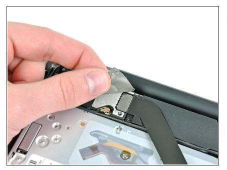
• Peel back the piece of EMI tape covering the AirPort/Bluetooth cable connector above the optical drive.
