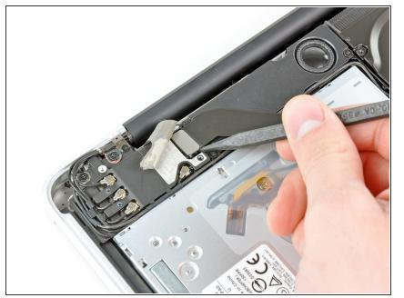
Use the tip of a spudger to lift the AirPort/Bluetooth connector off of its socket on the AirPort/Bluetooth board.
