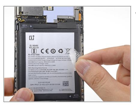
Peel the clear pull tab up from the battery.
