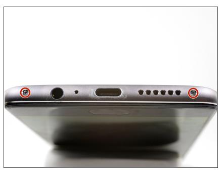
Remove the two 2.6 mm T2 screws from the bottom edge of the phone.
