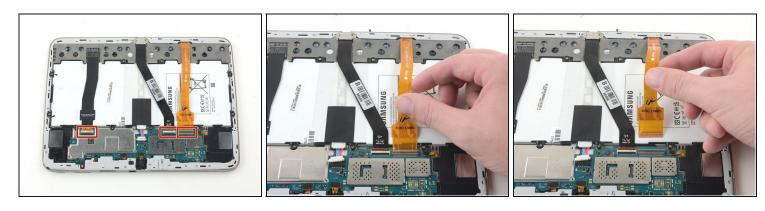
• Remove all three ribbon cables by gently pulling the cables away from the ZIF connectors.
