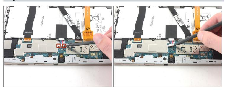
• Use the pointed end of a nylon spudger to pry the two battery connections away from the motherboard.
