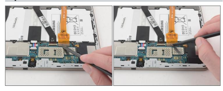
• Use the flat end of a nylon spudger to pry up the **brown** plastic tab securing the orange ribbon cable.
