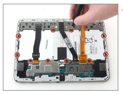
Use a Phillips #000 screwdriver to remove the ten 3mm screws securing the battery to the chassis.
