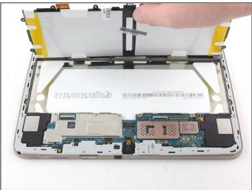
• Lift with a nylon spudger to remove the battery.
