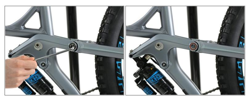
• Use a 6mm allen key to remove the stud bolt at the left side of the seat strut hinge.
