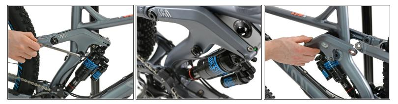
• Use a 6mm allen key to loosen the shaft of the rocker bearing on the right side of the frame.
