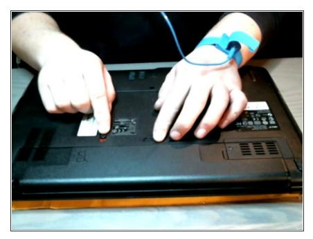
Make sure your computer is off and remove the battery with the security tabs shown in the picture
