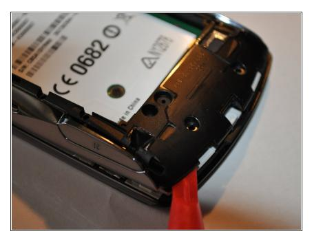
Using a plastic prying tool, go around the outside of the phone releasing the plastic clips.
