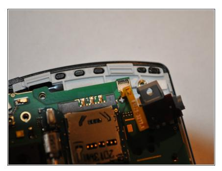
Remove the headphone jack by carefully moving the dark plastic clip on the connector to 90 degrees
