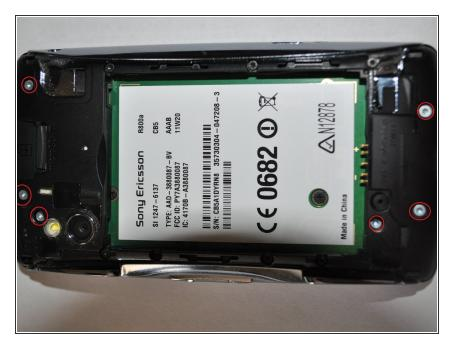
Remove the 6 silver torx screws marked in red
